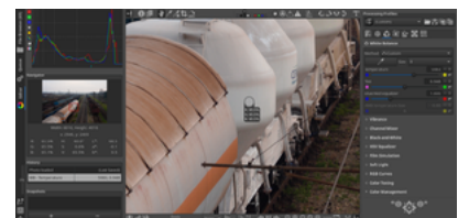
Picking the white balance off the side of this tanker, which we know to have been the whitest object in the scene, adjusts the colors across the whole image such that the RGB levels in that spot are now equal.
