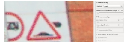
A good image to test the demosaicing algorithms on. Zoomed in to 800%, you can clearly see that VNG4 is not a good choice for this Pentax K10D raw file, as there are dots where there should be none, and the detail of the wall's brickwork (the orange part on the right) is all washed out.
